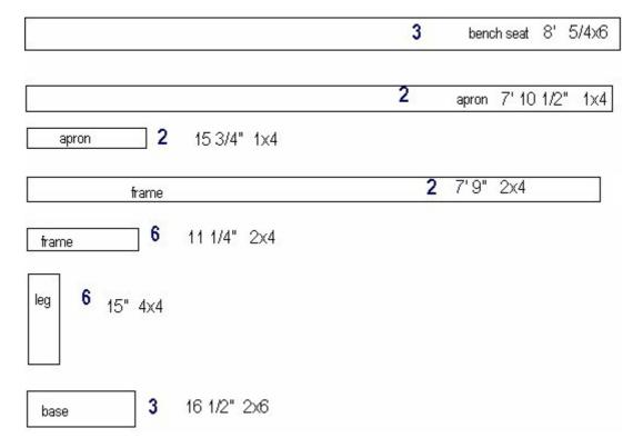
Start by building the 2x4 frame that will support the top and the legs. This is a simple box made of 2x4s. Cut 2 boards 7'9" each, and cut 6 boards 11 1/4 inches long. Use a 4x4 to gauge the distance between the two center boards since the center legs will fit between these two. Nail them all together using 16 penny galvanized tiwist or ring nails.
