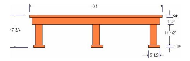
Now, flip the bench over upside down again, and attach the 1x4 apron boards to the 2x4 frame all the way around. Miter the ends by cutting them at a 45 degree angle. I gave you the sizes, in the cutting list above, but it helps to make these cuts after measuring the actual dimensions, to assure a nice clean fit. Attach the apron boards using 8 penny galvanized finish nails.
